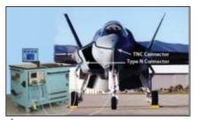
Fig. 5 An HPCC-3000 system measuring aerospace cable assemblies.
