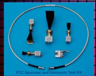
FCC Spurious and Harmonic Test Kit for use with popular Spectrum Analyzers. Each kit contains four mixers providing continuous coverage from 40 to 220 GHz. Each mixer is equipped with an appropriate horn antenna for accomplishing the FCC desired radiated spurious level measurement. Shown with optional diplexer and cable.
