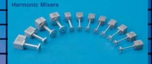
Harmonic Mixers Use with popular Spectrum Analyzers to achieve millimeter wave spectrum analysis. Mixers are available for all waveguide bands from 18 to 325 GHz. LO/IF diplexers are available for most modern spectrum analyzers. Measured conversion loss data supplied with emulation of most modern spectrum analyzers for WR-42 through WR-10.
