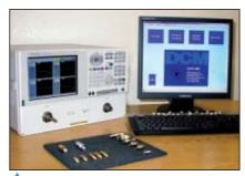
Fig. 1 DCM COAX-3000 system with modeled adapters and de-embedding module.
